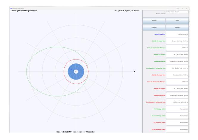
The red satellite is in circular orbit at an altitude which makes the satellite clock stay in sync with UTC.
