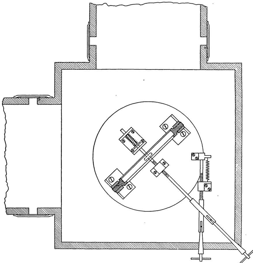
FIG. 2.—Details of corner box and mirror mounting
