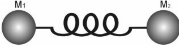
Figure 4: A pair of masses joined by a spring can be viewed as the simplest conceivable detector.
